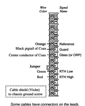
Cut off the connectors, skin and tin the leads and then wire to the screw terminals on the boards
